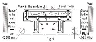
(2) Open a piping hole with the diameter of 2 3/16inch on the selected outlet pipe position. In order to drain smoothly, slant the piping hole on the wall slightly downward to the outdoor side with the gradient of 5-10°. (As show in Fig. 2)
