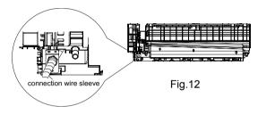
(3) Remove the wire clip; connect the power connection wire to the wiring terminal according to the color; tighten the screw and then fix the power connection wire with wire clip. After finishing wiring, clamp the grounding wire (yellow-green wire) into the wire-crossing groove (As show in Fig. 13), in order to avoid pressing the wire when closing the electric box cover. (As show in Fig. 13)
