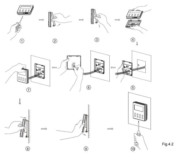
Fig.4.2 shows the installation steps of the wired controller, but there are some issues that need your attention.
